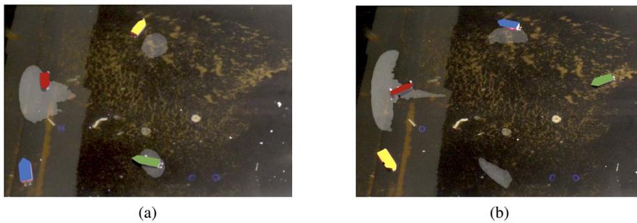
Fig. 15: Robotic boats tracking dynamic process in water tank. The dynamic process is shown in white, and robots in blue, red, yellow, and green. (a) Robots assume positions based on the initial POD basis. (b) Robots switch positions after collecting sensor measurements and updating their models.
